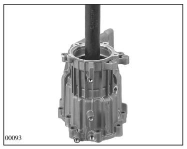
Using drift 5x46 002 259 in the mandrel press, force needle roller sleeve 36.130 into the transfer box housing 36.010 and secure with snap ring 36.150.
