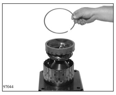
Disengage the snap ring and the divided planet carrier I from ring gear I with ring gear II.
