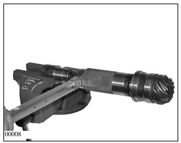
Screw locknut 35.040 with fixture 5x46 002 174 on to the pinion shaft and caulk into position.
