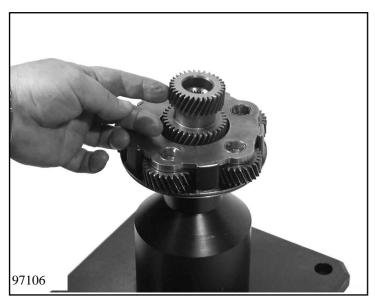
Lift planetary gear set (I and II with ring gear III) away from the fixture. Place planet carrier III 42.010 on the fixture and insert sun wheel 32.360.
