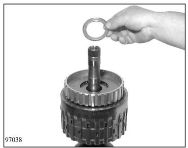
Lift off the axial needle roller bearing.
