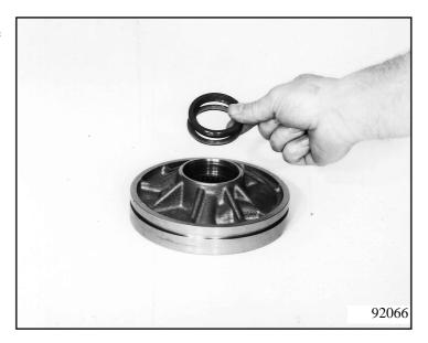
Press out the sealing ring with the needle roller bearing in the mandrel press. The diameter of the pressure pin is 42 mm.
