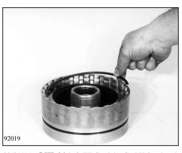
Disengage the snap ring and remove the entire disc set of brake F
