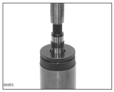
Use the puller 5x46 032 010 (Rollex 32010x1), tool 5x46 000 530 and the hydraulic press to press the bearing inner race off the pinion shaft.
