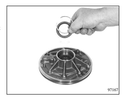
Press in sleeve 10.010/190. Pull on new O-ring 10.014. Lightly grease the pump gear and pump ring gear before assembly. After that, assemble pump such that one mark is visible at the pump ring gear and
