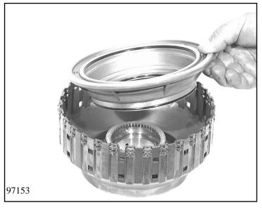
Pull two O-rings 72.030, 72.040 and sealing ring 72.050 on to piston B 72.020.
