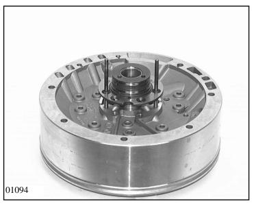
Heat intermediate plate 10.020/110 to app. 70° C with a hot-air blower. Screw 2 locating pins 5x46 001 007 into intermediate plate.
