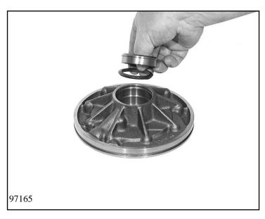
Add parts to pump 10.010; first insert sealing ring 10.010/140 into the pump housing, then press down needle roller bearing 10.010/150 in the mandrel press with installation drift  $5x46\ 000\ 954$ .
