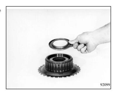
Insert the entire freewheel into brake F while turning it. Then engage snap ring 77.130 with installation tool 5x46 000 892 or by hand.
