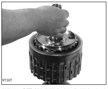
Place planetary gear carrier on the planet carrier while turning it.
