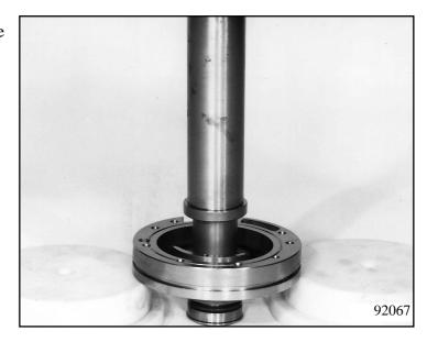
Undo 5 countersunk screws, heat the housing of the stator shaft to approx. 70° C and drive the stator shaft out of the intermediate plate with a plastic-faced hammer.
