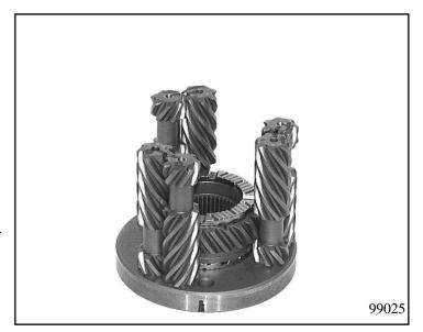
When looking clockwise, the first planet wheel of each pair has the tooth gap at the top. Mesh the planet wheels together and with the front sunwheel.
